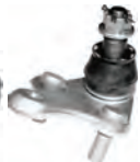
TO1918 Lower Ball Joint (Ø17.5)
