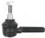
LR1010 Outer Tie Rod End (Ø15*Ø17.5/M12*1.5)
