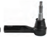
CH1014 Outer Tie Rod End (Ø13.1*Ø18.1/M16*1.5)
