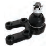
SS1911 Lower Ball Joint (Ø17.55)
