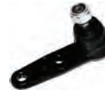
CH1911 Lower Ball Joint (Ø14.9)
