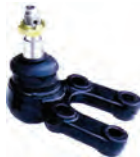
MH1912 Lower Ball Joint (Ø17.6)
