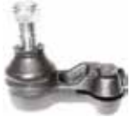
DA1010 Outer Tie Rod End (Ø13*Ø15.3/M16*1.5)
